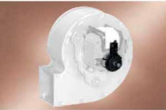
The signal transmitter SG2 is an impulse transmitter suitable to be connected to EM30 and KM motors. 12 square impulses per rotation of the motor shaft are formed by means of a 24-pole, plastic-bonded ferrite magnet ring, in connection with a Hall-IC.
